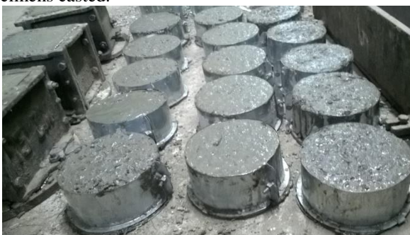
Fig. 2.2: Disc specimens for drop weight test and cubical specimens for compressive strength test.
