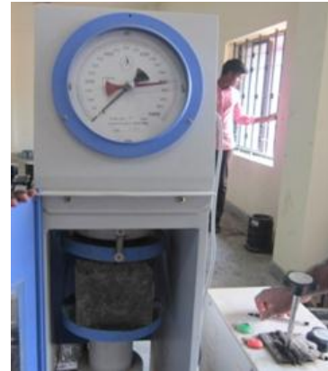
Fig. 3: Compressive strength test
