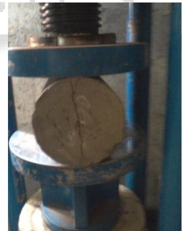
Fig. 4: Split tensile strength test
