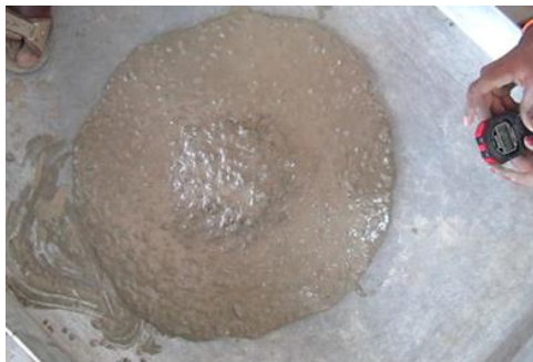
Fig. 1: Slump Flow & T50 Test
