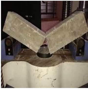
Fig. 6: Failure of beam without Reinforcement
