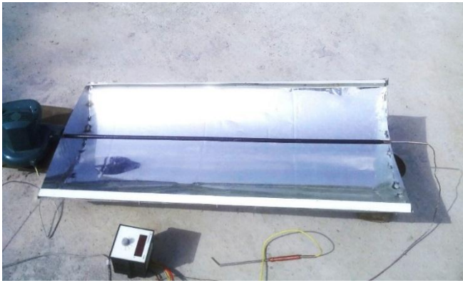
Fig. 4: Experimental setup of parabolic trough collector solar air heater
