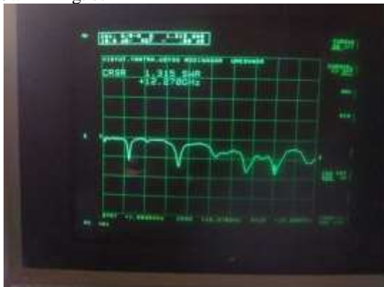
Fig. 7: Return Loss of Fabricated Proposed Antenna
