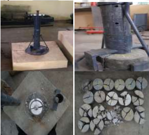
Fig 1: Impact testing of specimens
