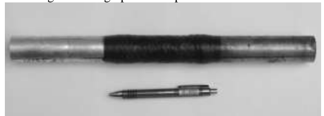
Fig 3: Photograph of the specimen Al-CFRP-Al
