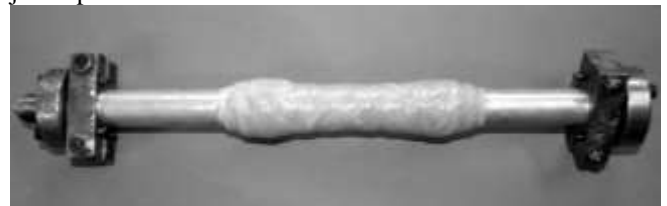
Fig. 9: Photograph of actual assembly GFRP sleeve specimen
