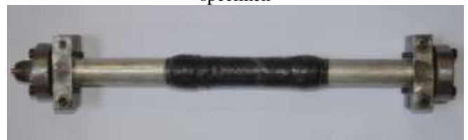
Fig. 10: Photograph of actual assembly CFRP sleeve specimen
