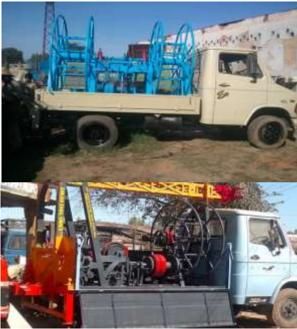
Fig. 6: Mechanically Actuated Motor Lifting Machine.
