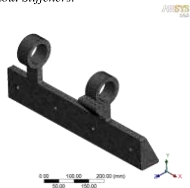
Fig. 8 Meshed Model (Scraper without Stiffeners)
