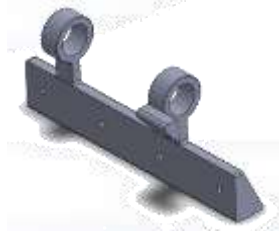
Fig. 2 Scraper without Stiffeners
