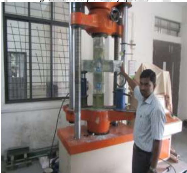
Fig. 4: Test setup glass specimen.
