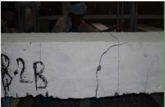
Fig. 7: Failure of Beam at Ultimate Load
