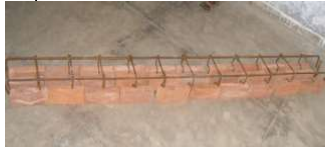
Fig. 1: Arrangement of Bricks with Reinforcement Cage
