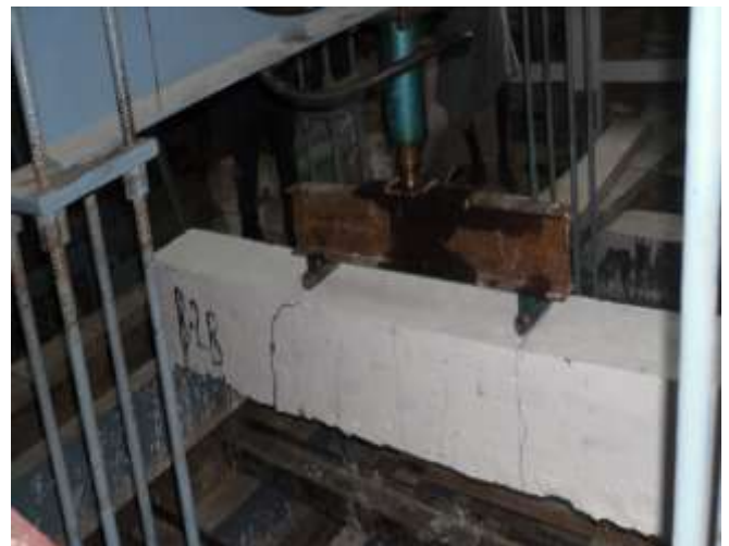
Fig. 9 Crack Pattern of 2nd group of beams
