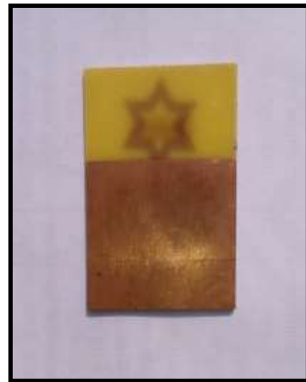
Fig. 6: Back view of fabricated Star shaped Fractal Antenna after 1 st iteration
