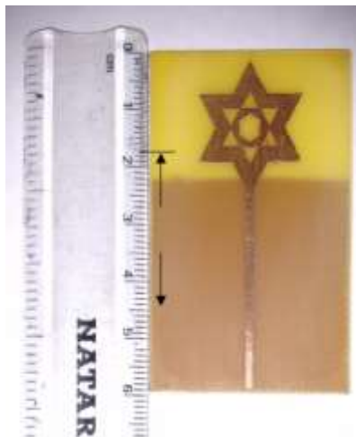
Fig. 9: Fabricated Star shaped hexagonal iterated Fractal Antenna after 2 nd iteration
