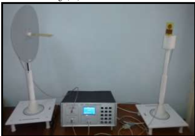
Fig 15: Antenna under measurement using antenna measurement system
