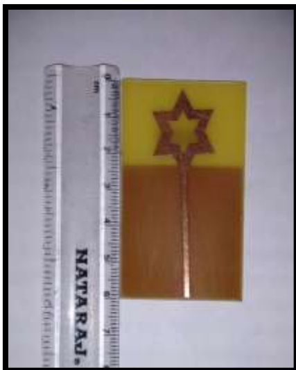
Fig. 5: Front view of fabricated Star shaped Fractal Antenna after 1 st iteration
