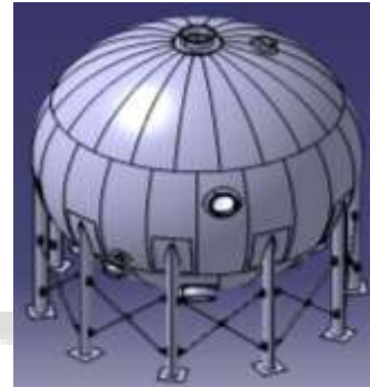
Fig. 2: Spherical pressure vessel assembly with cross bars
