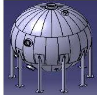
Fig. 1: spherical pressure vessel assembly
