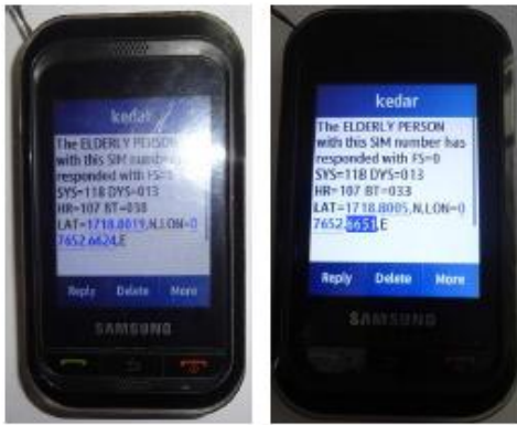
Fig. 7: Photograph of a Mobile Phone with SMS sent by the Wearable Unit
