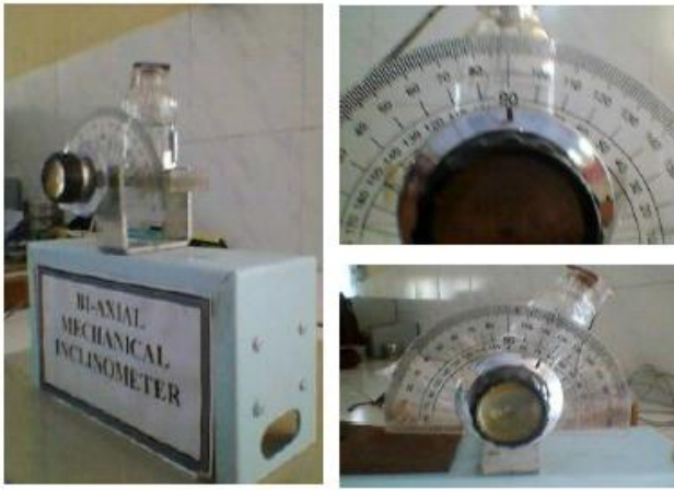
Fig. 4: Shows Bi-Axial Mechanical inclinometer for fall angle measurement & right image shows 24° Fall Angle
