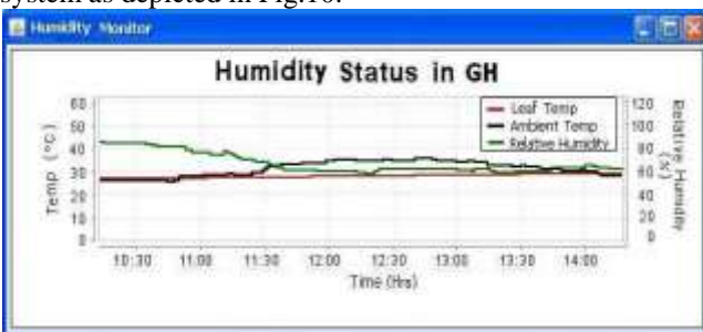
Fig. 10: Simultaneous plotting of temperature and humidity parameters at PCN system
