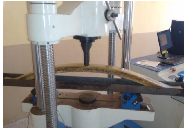
Fig. 4: Load applied on composite leaf spring
