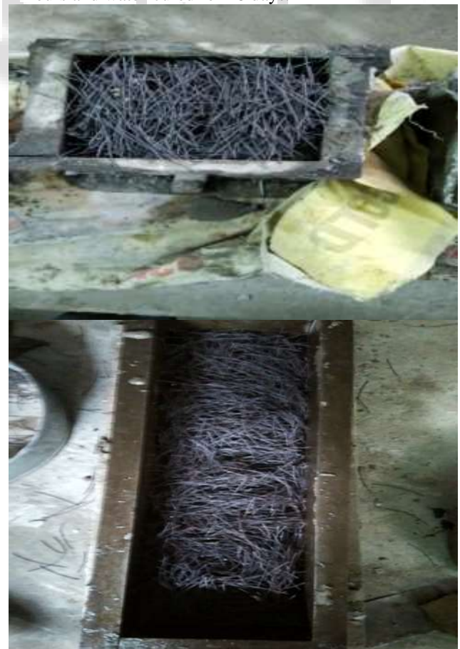
Fig 1 Placement of Steel Fibres in mould
