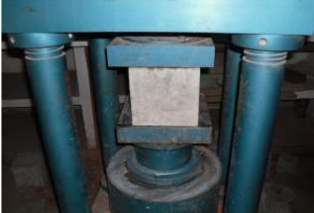
Fig. 2: Compressive Strength Testing Machine
