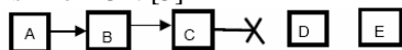
Fig. 5: Node C is unable to forward a packet from A to E over the next node D[3]
