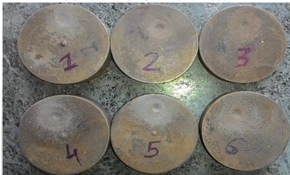
Fig. 2: Workpiece Material after EDM
