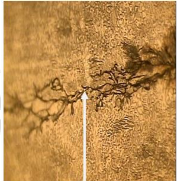
Fig. 6: Cracks in Nugget at 500 X In ASS 304 & ASS 202
