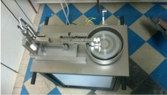
Fig. 2: A Photograph View of the Pin-On-Disk Type Wear Testing Machine
