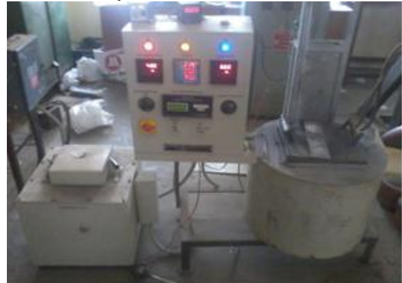
Fig. 1: A Photographic View of Stir Casting Machine
