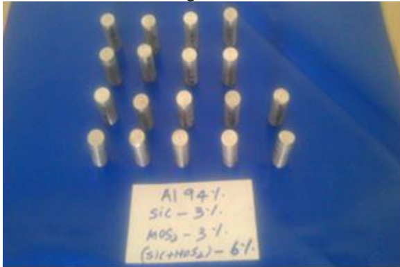
Fig. 3: The Photographs View of the Wear Tested Specimen.
