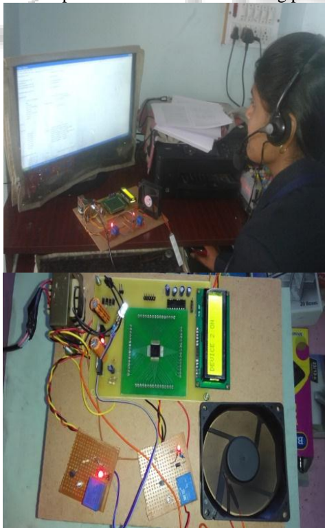
Fig. 5: Hardware Of "Home Appliance Control Using Speech" System
