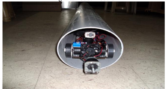
Fig. 12: Mobile Robot inside Pipeline
