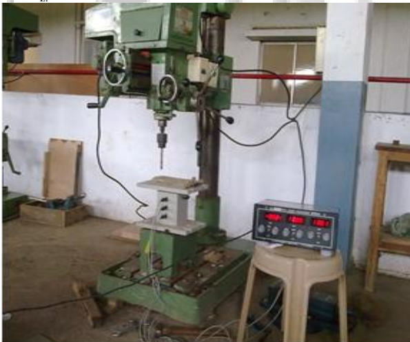
Fig. 2: Drilling and measuring the force for sandwich composite
