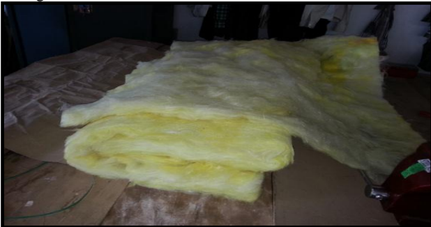
Fig. 3: Glass wool as wick material
