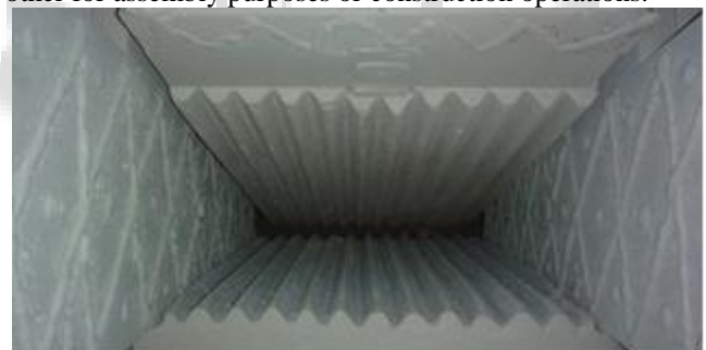
Fig. 4: Picture Showing Corrugated Cast Steel Jaw Plate
