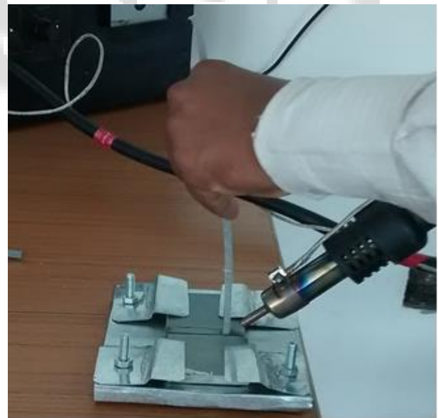
Fig. 1: Hot Air Welding Operation Performing in Lab Weld beads at different combination of welding parameter obtained are shown below:
