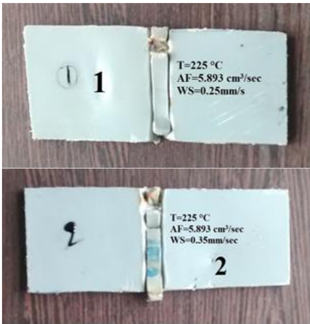
Fig. 2: Weld Bead Obtained using Different Combination of Input Parameter
