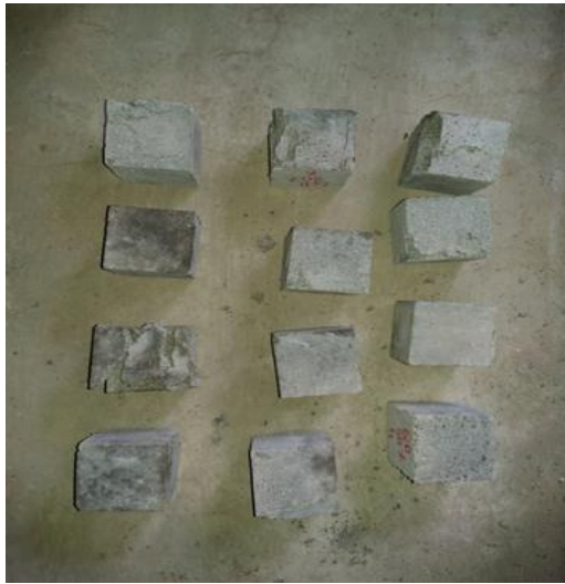
Fig. 4.5: Failure pattern of cubes
