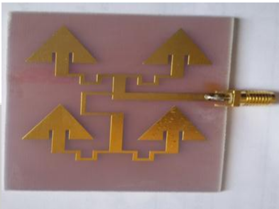
Fig. 9: Fabricated 2x2 TMSA
