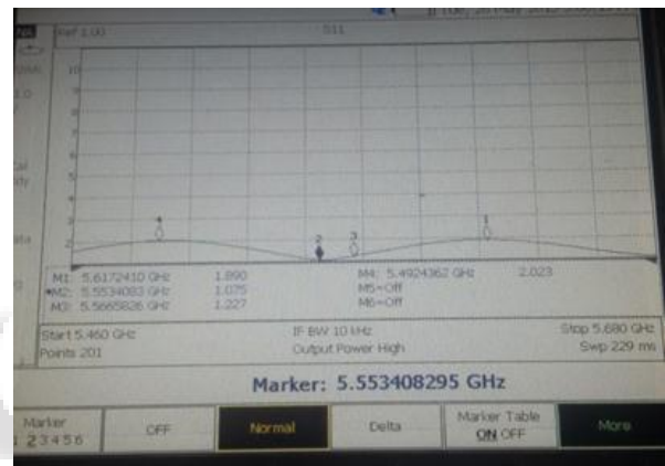
Fig. 12: VSWR of fabricated 2x2 TMSA
