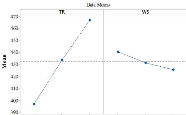
Fig. 4: Graphical representation of main effect of Tool rotational speed (TR) and Welding speed (WS) on Maximum Temperature during friction stir welding of Aluminium Alloy AA-7075.
