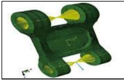
Fig. 2: Model with rectangular slot component is subjected loading and boundary conditions
