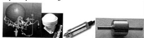
Fig. 6: The cold-gas micro-propulsion system of NanoSpace. (most left- System; second left- MEMS thruster module; second right- MEMS pressure sensor; most right- MEMS isolation valve)
