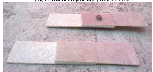
Fig 7: chopped strand mat lap joint
