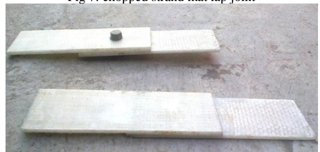
Fig 8 : Bi-Directional fly lap joint
