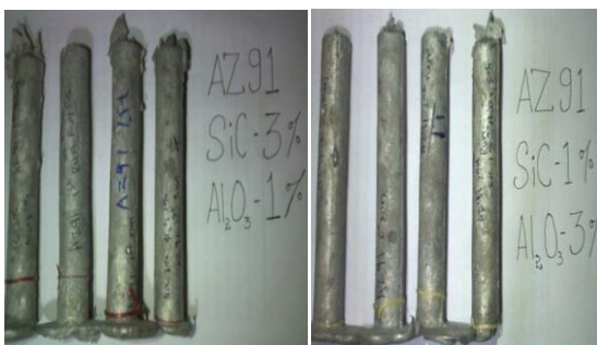
Fig: Prepared reinforced Mg-9Al-1Zn
