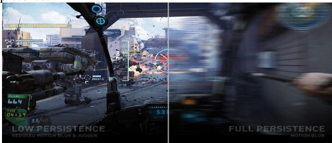
Fig. 1: Example of low persistence OLED
