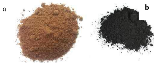
Fig. 2: (a) Dried and grinded biosorbent (b) Activated biosorbent
