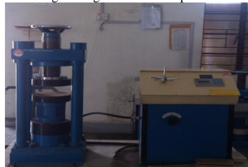
Fig. 8: Set up of Compressive Testing Machine
