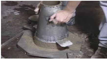
Fig. 9: Slump cone test for Workability Source : S.N.P.I.T. & R.C., Umrahk
