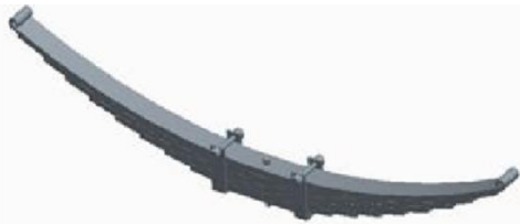
Fig. 1: Solid model of a leaf spring created in Creo software
