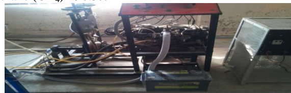
Fig.1 Four stroke multi cylinder petrol engine test rig with rope brake dynamometer
