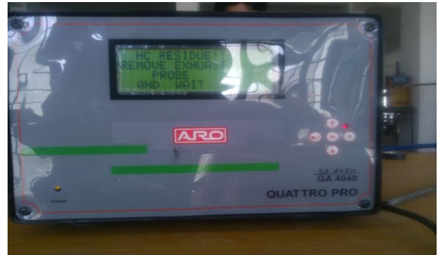
Fig. 3: Exhaust gas analyzer
