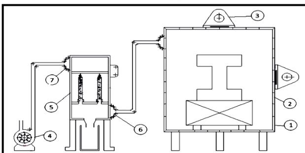
Fig. 1: General diagram of shot blasting machine
