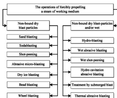
Fig. 3: Classification of Shot blasting process
