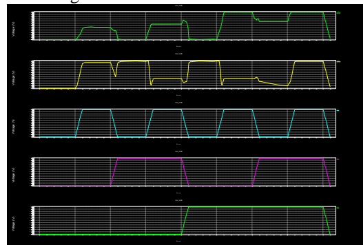
Fig. 2: output Waveform of 16T full adder
