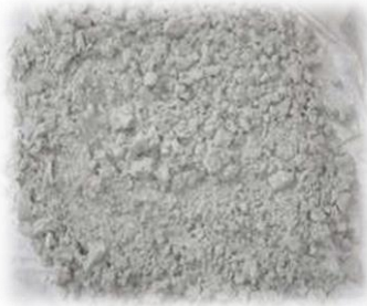
Fig. 2: Hypo Sludge Source: -engineeringcivil.com
