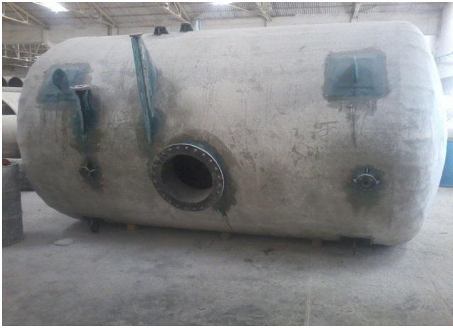
Fig.10: Final model of FRP Pressure vessel
