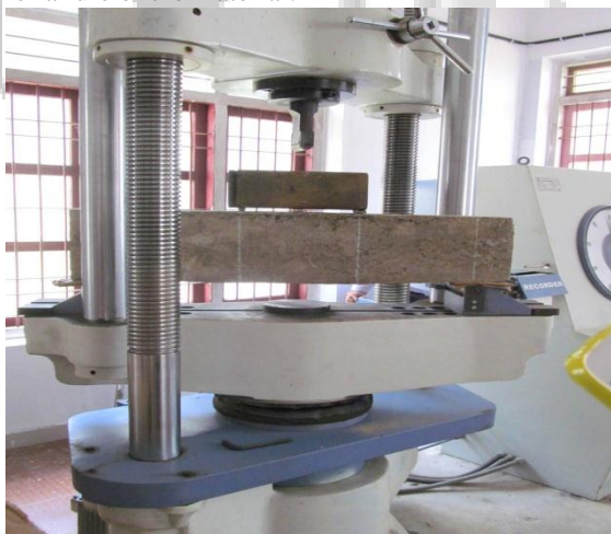
Fig. 6: UTM test setup for 4-point flexure
