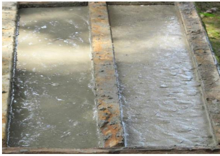
Fig. 5: Casted beam specimens
