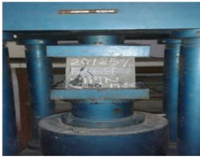
Fig 5.3: Compressive strength test procedure and loading condition
