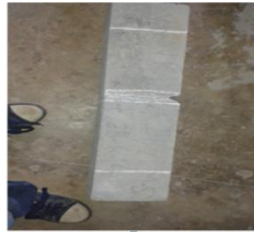
Fig. 5.6: Flexural Strength Test of prism unloading condition
