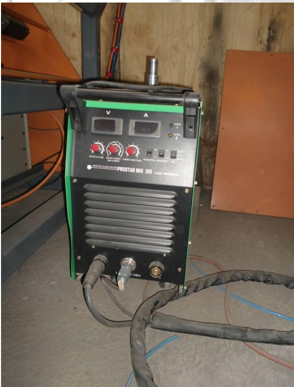
Fig. 2: Gas metal arc welding Set up
