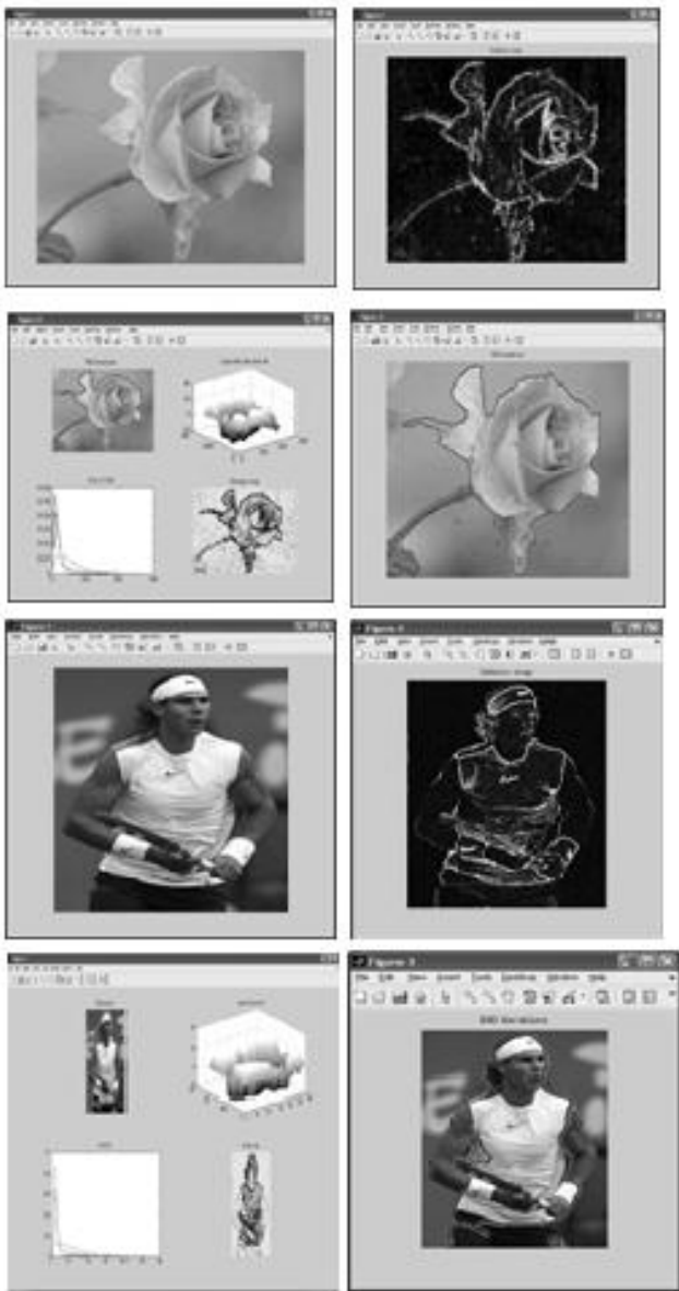
Fig. 2: (a) Input Image (b) Saliency Map (c) Iteration, Lipschitz function, Energy Map (d) Low DOF image segmentation
