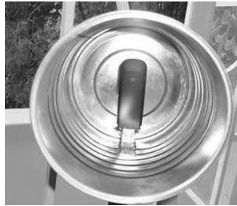
Fig (2), (3), (4) Different methods for Practical implementation of parabolic foil with dongle for increasing signal strength
