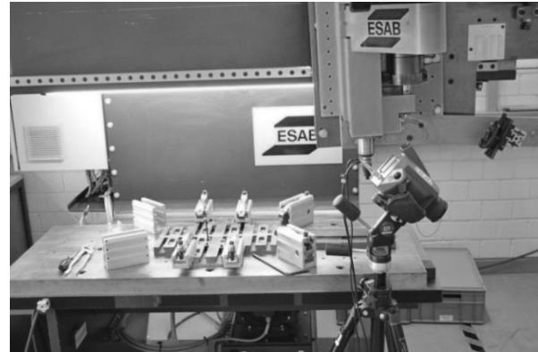
Fig. 3. Layout setting for thermal camera measurements
